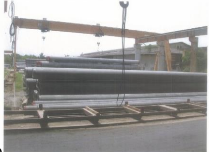
8. after demolded, piles are sent to stock yard.
