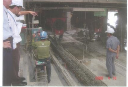
Pouring concrete (C50) inside the mold.
