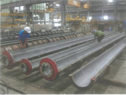
Fixing the upper mold (after pouring concrete).
