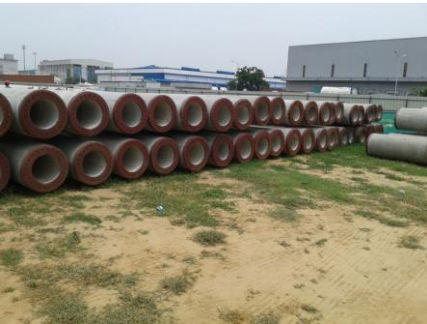
8. after demolded, piles are sent to stock yard.
