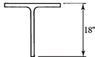
Structural Tee: WT, ST, or MT (WT18 × 105 shown)
